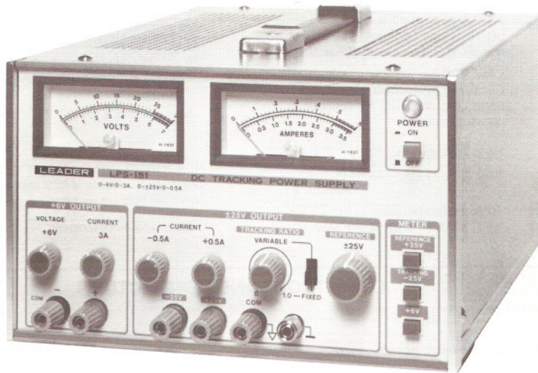
Figure 1-1. DC Tracking Power Supply
